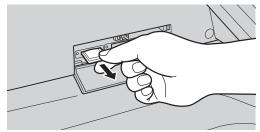
Do not remove the SD Memory Card while the Access Indicator is flashing.
